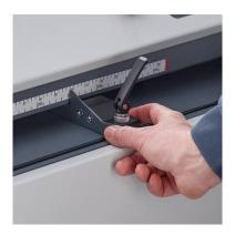
Measurement scale enables the material width to be easily adjusted to the extent it is required for box lining
