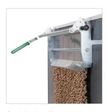
**Cushioning flap** to adjust the cushioning volume of the output material to fill void in the box more efficiently
