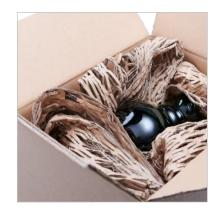
Fill material using of packaging material to fill up voids between products and box walls
