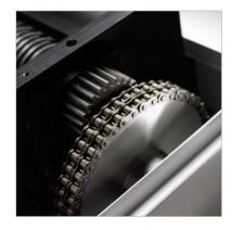
Robust construction due to the metal chains, gears and bearing plates, ensures a long operation life of the machine
