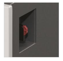
Recessed main switch with the ability to secure it with a padlock to prevent unauthorized use
