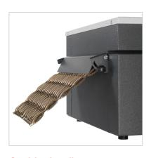
**Cushioning flap** to adjust the cushioning volume of the output material
