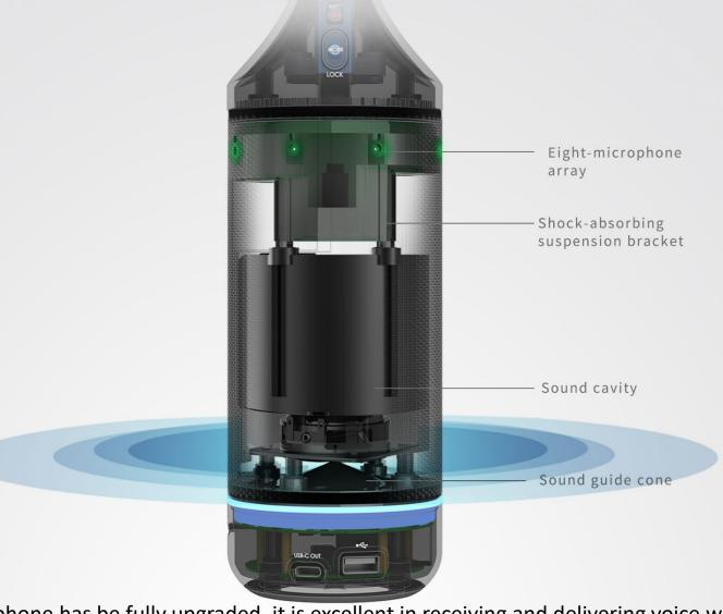
The quality of speaker and microphone has be fully upgraded, it is excellent in receiving and delivering voice, with up to 5.5 meters radius coverage, the effective use area is nearly 2 times higher than the previous generation . Omni-directional Audio System
