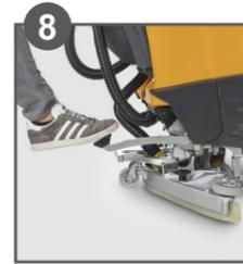
8 Lower brush units by using the manual lever (by foot)
